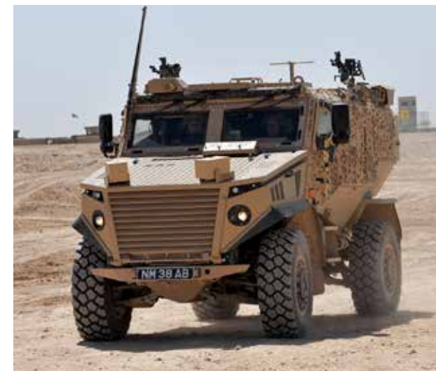
New hybrid electric drive Foxhound and Jackal vehicles for the British Army to improve stealth capability and environmental impact, working in conjunction with General Dynamics, Magtec and Supacat.
